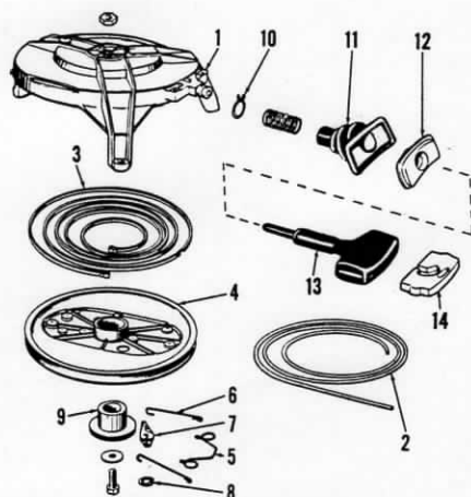
Fig. OM7-15—Exploded view of starter typical of all models. Minor differences will be noted on examination.
